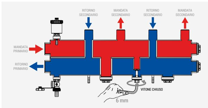
Close the bonnet completely to close the communication path between delivery and return circuits and transform device back into a boiler room manifold.
