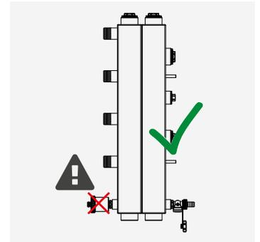
**⚠ WARNING.** For vertical or upside down installations, do not install the air vent valve; replace it with a 1/2" M plug if necessary.
